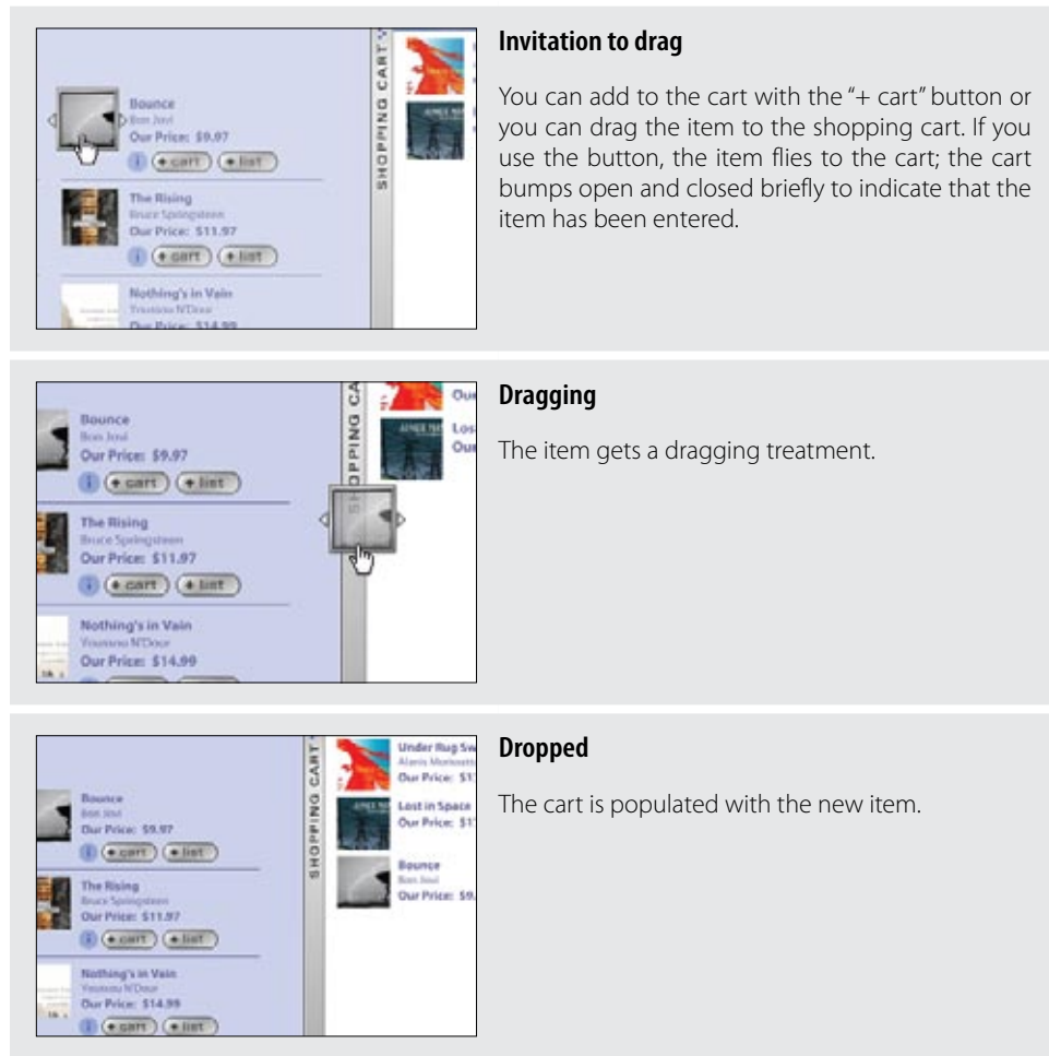
Figure 2-34. This Laszlo shopping cart demo uses both drag and drop and a button action to add items to its shopping cart
